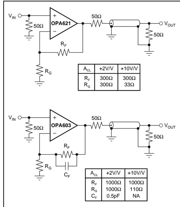
FIGURE 3. Application Circuits for OPA621 and OPA603.
