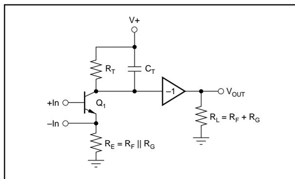
FIGURE 2. Current-Feedback Amplifier Simplified and Reconfigured for Analysis.
