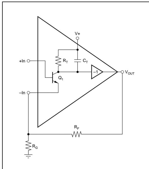
FIGURE 1. Current-Feedback Amplifier Simplified for AC Analysis.
