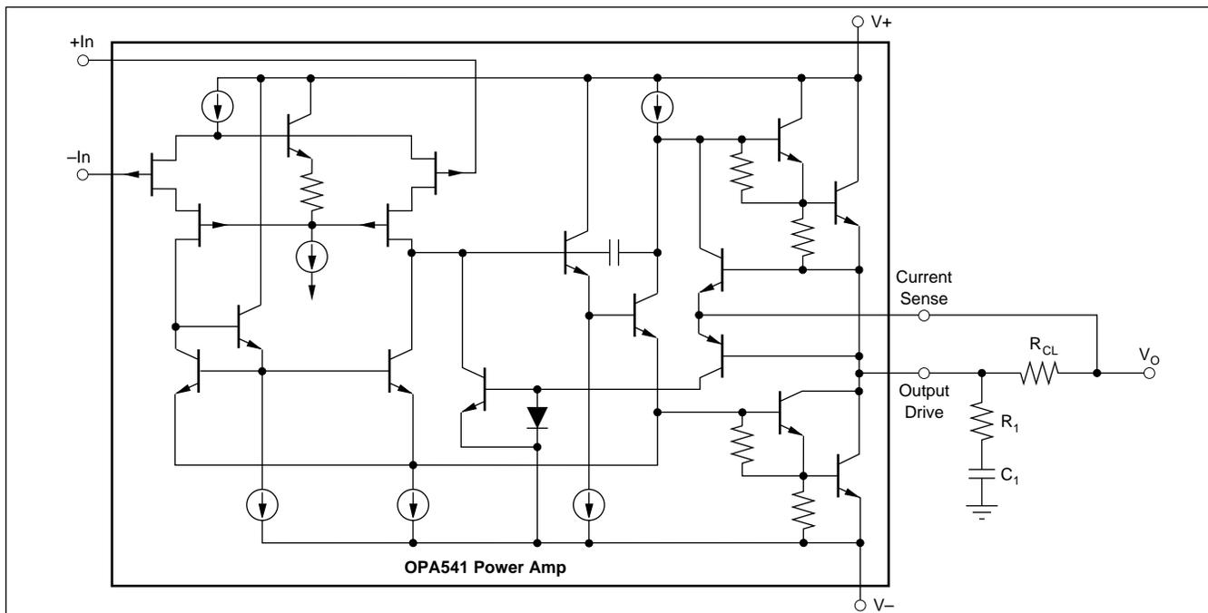
FIGURE 1. An R<sub>1</sub>, C<sub>1</sub> network can be added to the OPA541 output to improve stability during current limit.
