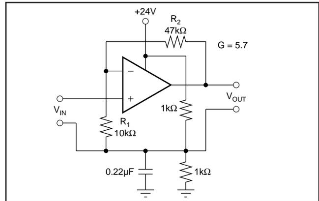
FIGURE 5. Even Though the Impedance of the Voltage Divider is in Series with  $R_1$  to Ground, the Gain of this Noninverting Circuit is Determined Solely by  $R_1$  and  $R_2$ . Since the input and output are referenced to the same floating ground, its impedance does not affect the voltage gain of the circuit.
