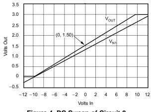
Figure 4. DC Sweep of Circuit 2
