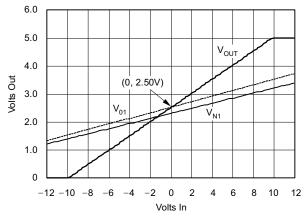
Figure 6. DC Sweep of Circuit 3
