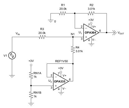
Figure 3. Circuit 2: Single-Supply/Single-Part
