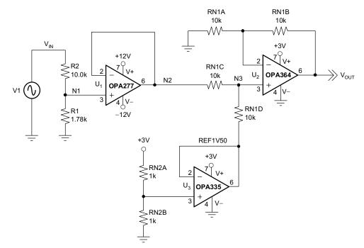
Figure 1. Circuit 1: Modular Design
