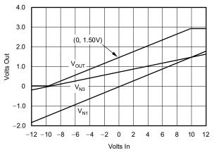
Figure 2. DC Sweep of Circuit 1
