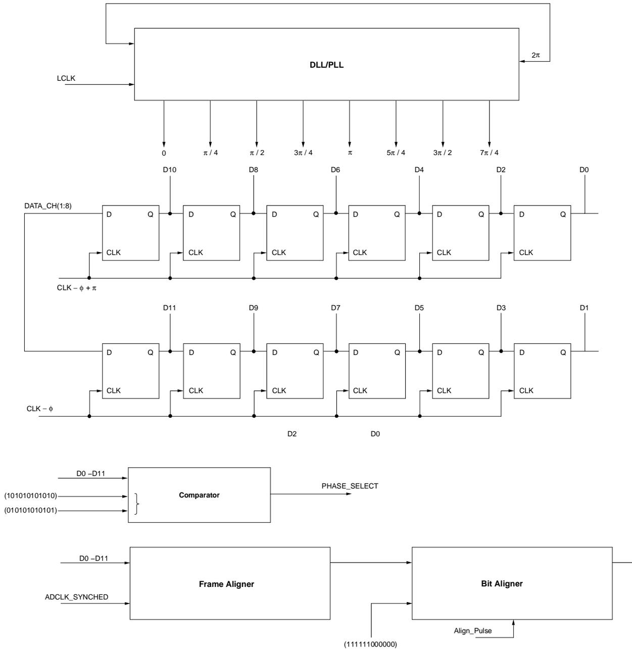
**Figure 3. Deserializer Architecture for Extending Receiver Capture Rate**
