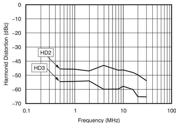
Figure 10. TxA Amplifier Transmitting While TxB Output is in Low-Impedance Mode: Harmonic Distortion vs Frequency Load
