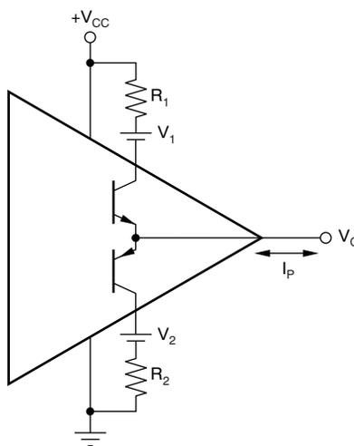
Figure 2. Output Voltage Headroom Model
