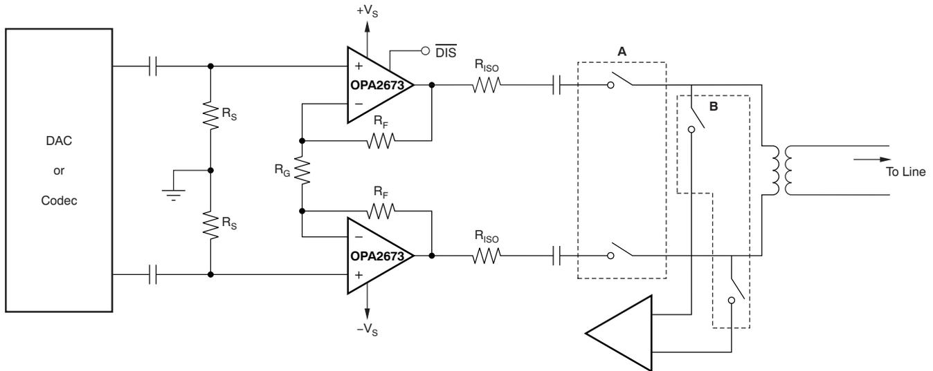
Figure 9. Complete PLC Line Driver Circuit
