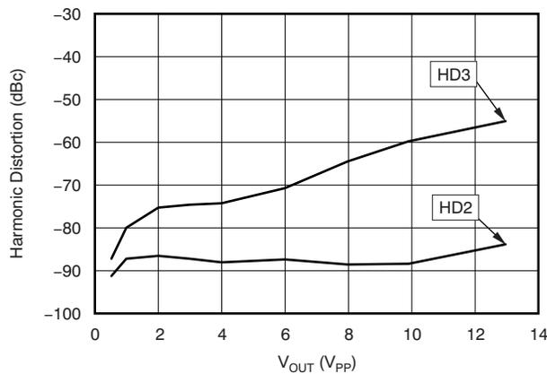
**Figure 14. TxA Amplifier Transmitting While TxB Output is Disabled: Harmonic Distortion vs Output Voltage**
