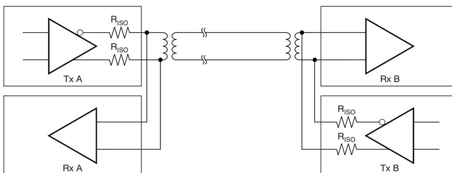
**Figure 8. Complete Signal Chain**
