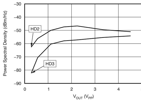
**Figure 11. TxA Amplifier Transmitting While TxB Output is in Low-Impedance Mode: Harmonic Distortion vs Output Voltage**
