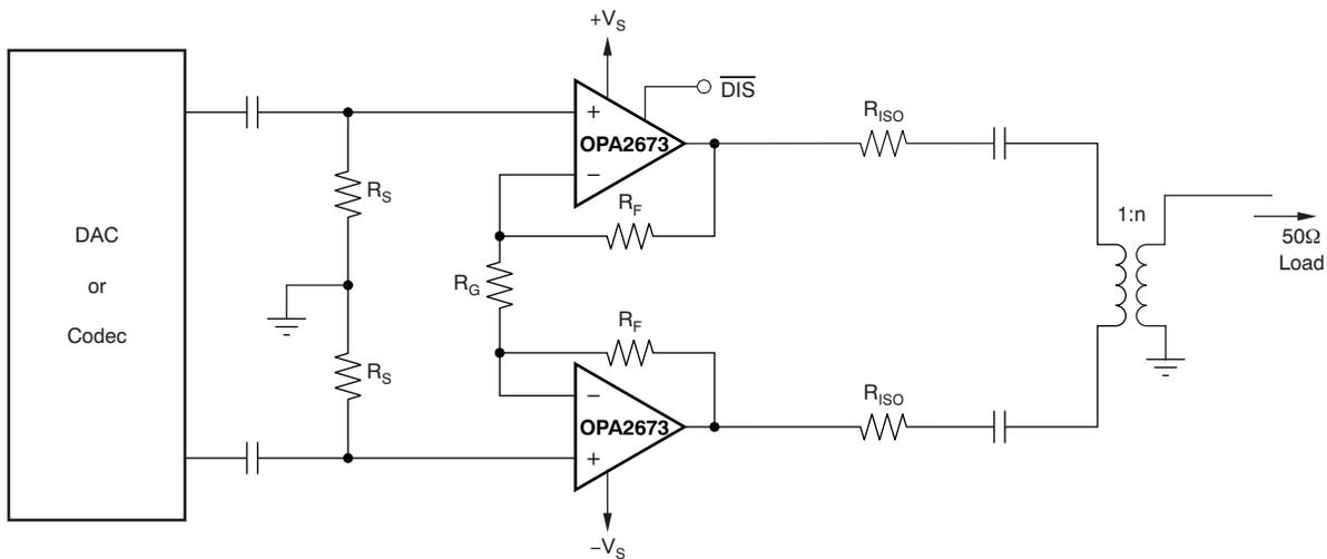
**Figure 3. Simplified PLC Line Driver**
