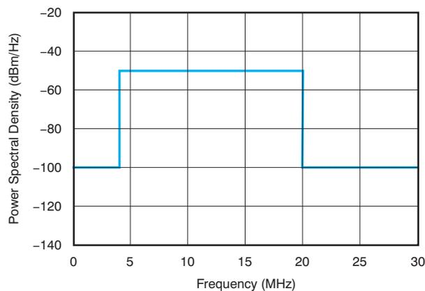
**Figure 4. Power Spectral Density Mask**
