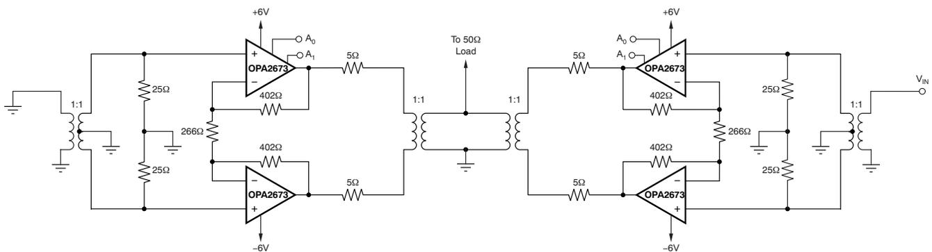
**Figure 12. TxA Amplifier Transmitting While TxB Output Stage is in Low-Impedance Mode: Circuit Configuration**
