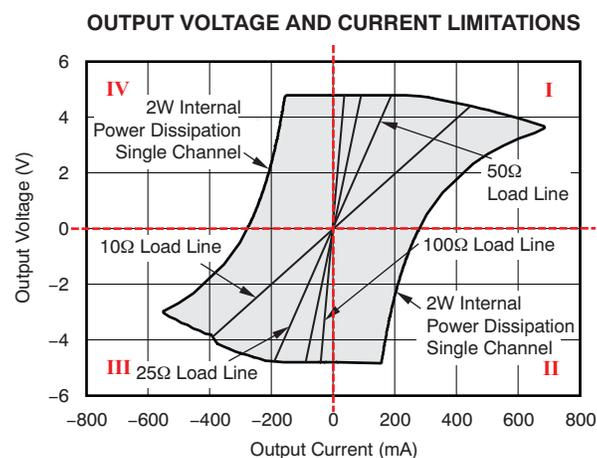
**Figure 1. Output Voltage and Current Limitations (OPA2673)**
