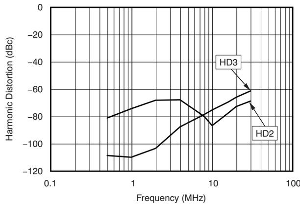
**Figure 13. TxA Amplifier Transmitting While TxB Output is Disabled: Harmonic Distortion vs Frequency Load**
