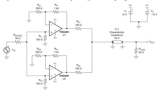
Figure 3 shows two THS3091 devices configured in a typical load sharing configuration.
