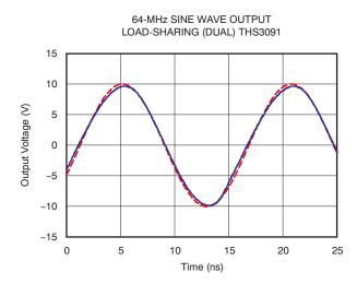
Figure 12. 64-MHz Sine Wave Output (Gain = 5 V/V, Signal Amplitude Referred to Amplifier Output), Two THS3091 Amplifiers in Load Sharing Configuration
