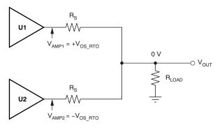
Figure 4. Simplified Load Sharing Circuit
