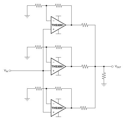
Figure 2. Load Sharing Conceptual Block Diagram
