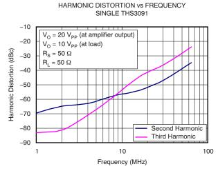
Figure 13. Harmonic Distortion vs Frequency, Single THS3091 Circuit Configuration
