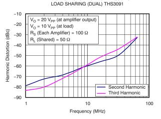
Figure 14. Harmonic Distortion vs Frequency, Two THS3091 Amplifiers in Load Sharing Configuration
