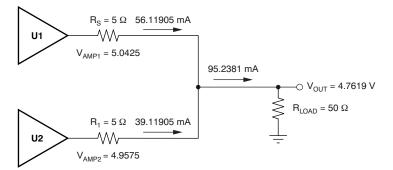
Figure 5. Example of Mismatched Amplifier Output Voltages Producing Unbalanced Amplifier Currents
