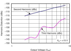
THS6182: G = -1 V/V, 1 kHz HARMONIC DISTORTION vs OUTPUT VOLTAGE
