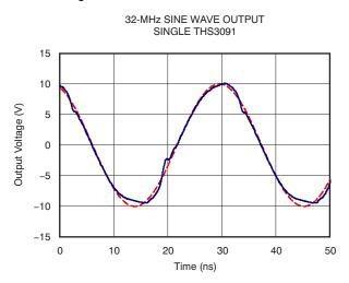
Figure 9. 32-MHz Sine Wave Output (Gain = 5 V/V, Signal Amplitude Referred to Amplifier Output), Single THS3091 Circuit Configuration
