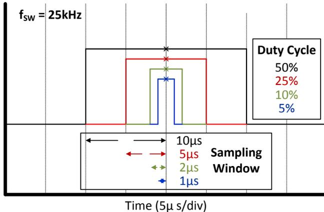
**Figure 2. Duty Cycle Impact On Settling Time**
