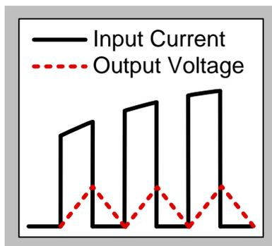
**Figure 3. Slew Rate Limited Output**
