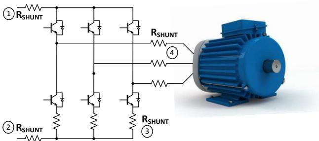
**Figure 1. Measurement Locations In A Three-Phase System**
