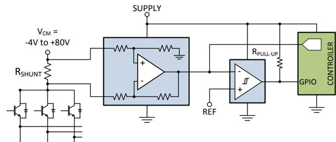
**Figure 3. High-Side Over-Current Detection**
