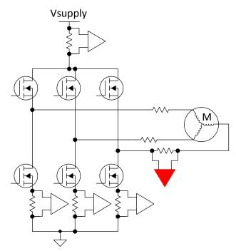
Figure 4. Inline Implementation of Current-Sensing Amplifiers (Only One Phase Shown)
