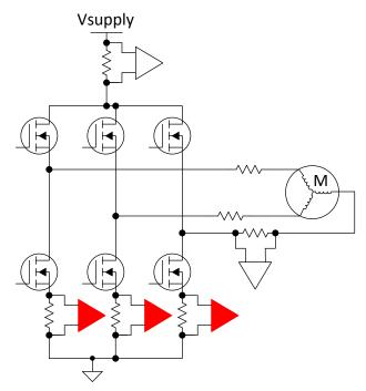
Figure 2. Low Side Implementation of Current Sensing Amplifiers
