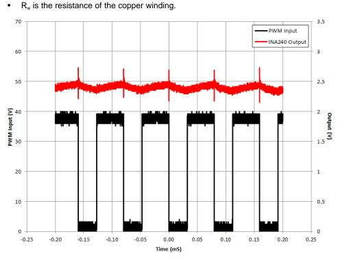
Figure 8. INA240 Output vs PWM Input
