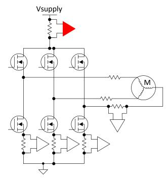
Figure 3. High Side Implementation of a Current Sensing Amplifier
