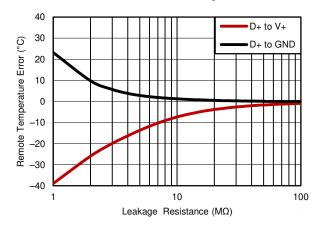
Figure 14. Leakage Resistance Effect on TMP468 Accuracy
