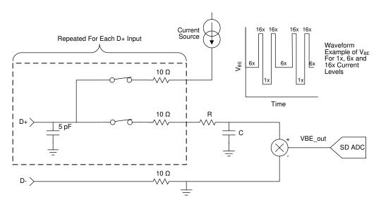
Figure 13. TMP468 Input Stage Simplified Schematic
