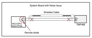
Figure 22. Isolating Noise Coupling Into Remote Transistor Traces
