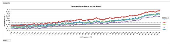
Figure 7. Example Data Set of TMP468 Temperature Error Using n-factor Correction Register Calibration
