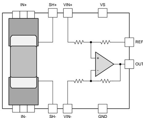
**Figure 3. INA250 Block Diagram with internal resistor connections**
