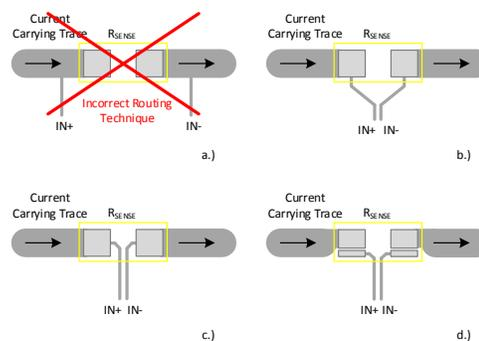
**Figure 2. Current Sense Resistor Layout Techniques**
