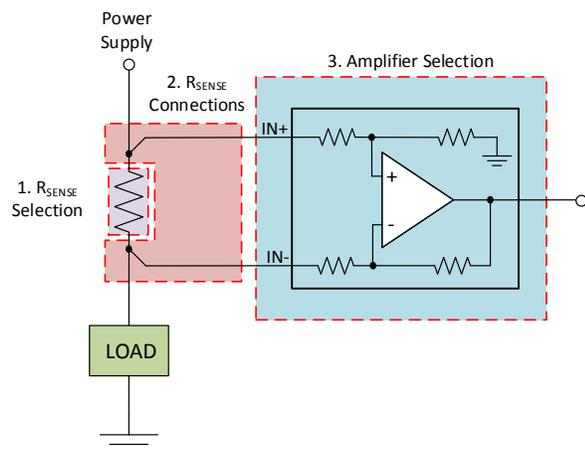
**Figure 1. High-Side Current Sensing with Shaded Error Sources**
