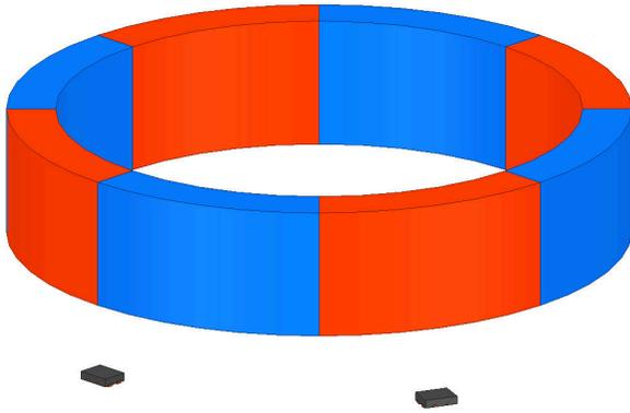
**Figure 3. Magnetic Incremental Encoder**
