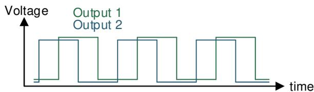
Figure 2. 2-Bit Quadrature Output
