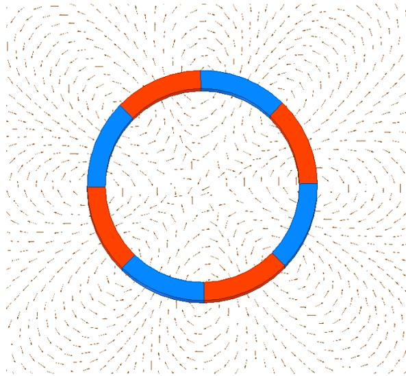
**Figure 4. In-Plane Magnet Field Vectors**
