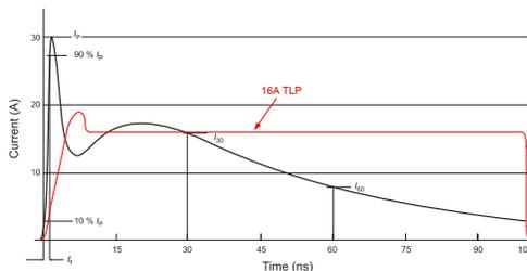
Figure 3. TLP vs. IEC61000-4-2 ESD Pulse
