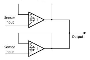
**Figure 5. Input Clamping Diodes**
