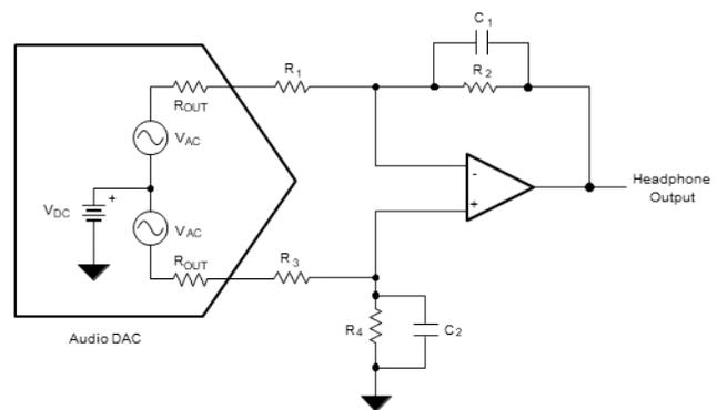
Figure 2. Audio DAC Output Circuit
