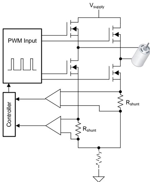
Figure 1. H-Bridge Motor Driver with Low-Side Current Sensing
