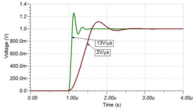
**Figure 3. Slew Rate Comparison**
