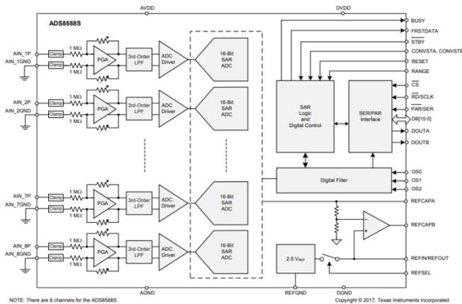
Figure 3. Simultaneous Sampling
