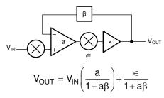
Figure 2. Circuit Diagram
