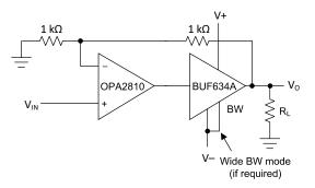
Figure 1. Composite Loop Using the OPA2810 and BUF634A
