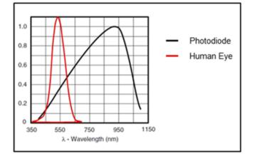
Figure 2. Typical Photodiode Response
