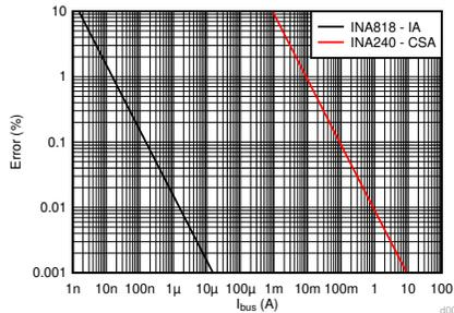
**Figure 2. Percent Error due to Maximum Input Bias Current vs Supply Bus Current**
