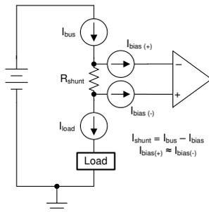
**Figure 1. Simplified Current Measurement Application Using a Shunt Resistor**
