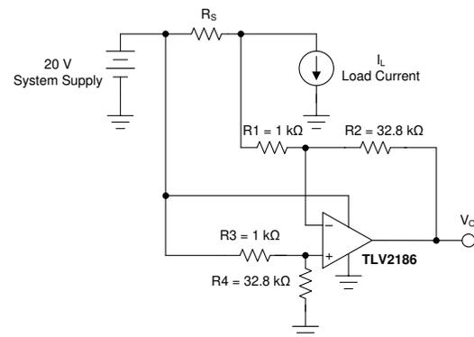
Figure 1. High-Side Current-Sense Circuit
