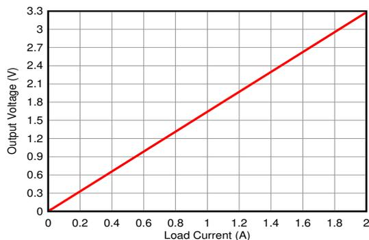
Figure 2. TLV2186 Output Voltage vs Load Current
