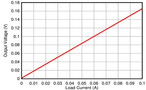
Figure 4. TLV2186 Output Voltage With Negative Supply Rail
