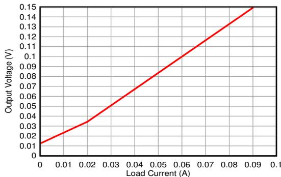
Figure 3. TLV2186 Output Voltage With Low Load Current
