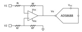
Figure 2. Front end Connected to ADS8688
