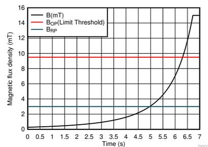
Figure 4. Magnetic Flux Density for End-of-Travel Detection
