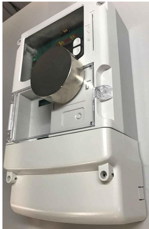
**Figure 1. Magnetic Tampering in Electricity Meters**
