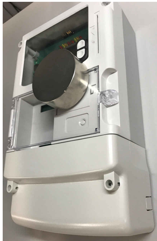
Figure 1. Magnetic Tampering in Electricity Meters
