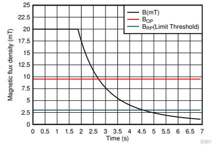
Figure 3. Magnetic Flux Density for Case Tamper Detection
