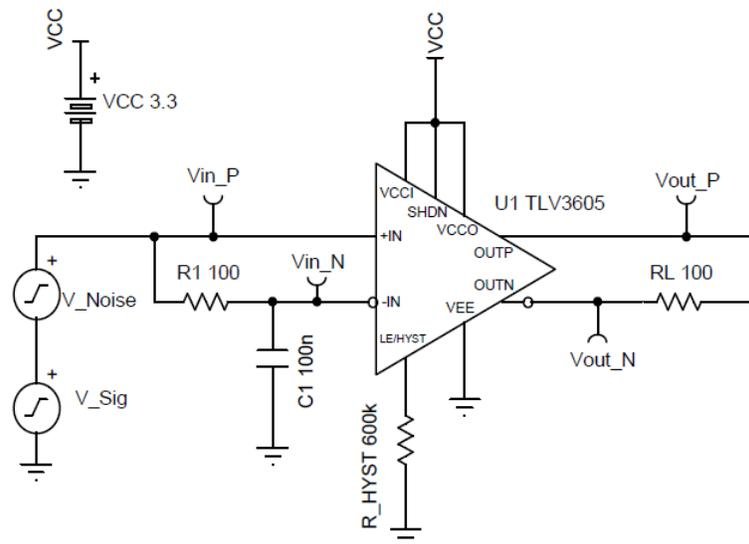
1. Set the non-inverting input of the comparator to the input data signal.
