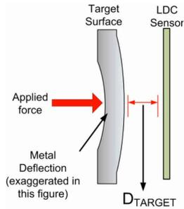
**Figure 2. Inductive Sensing Technology for Touch Buttons**
