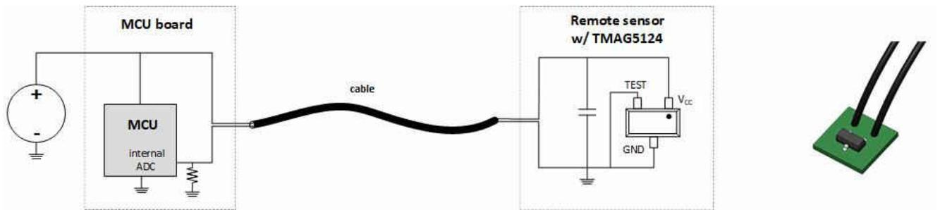
**Figure 3. TMAG5124 Two-Wire Connection and Small PCB Implementation**
