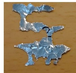
Figure 3-12. Aluminum Foil After Ultrasonic With De-ionized Water
