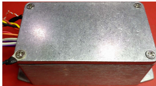
Figure 3-7. Aluminum Box for Shielding High-Impedance Node From EMI
