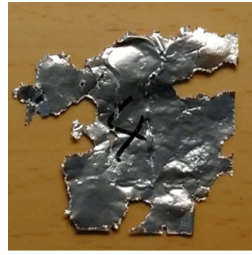
Figure 3-13. Aluminum Foil After Ultrasonic With Tap Water
