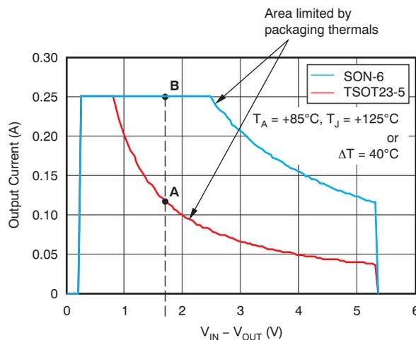
**Figure 3. Thermal-Safe Operating Area for +85°C in Ambient Air**
