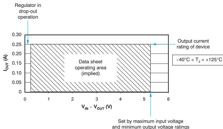
**Figure 1. Implied Operating Area of a Linear Regulator Based on Data Sheet Specifications**
