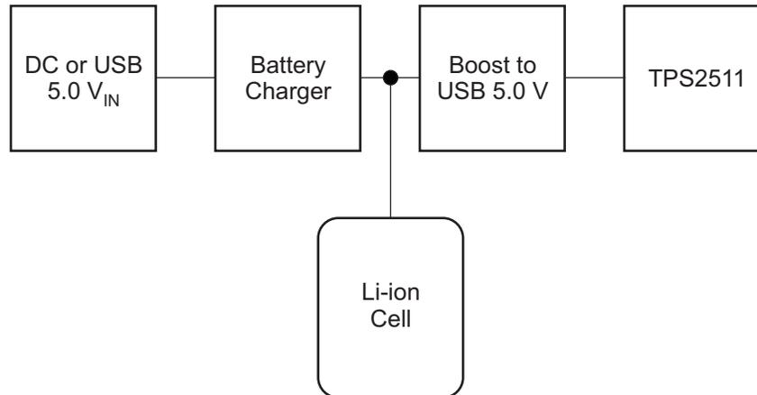
**Figure 3. Basic Power Bank Block Diagram**
