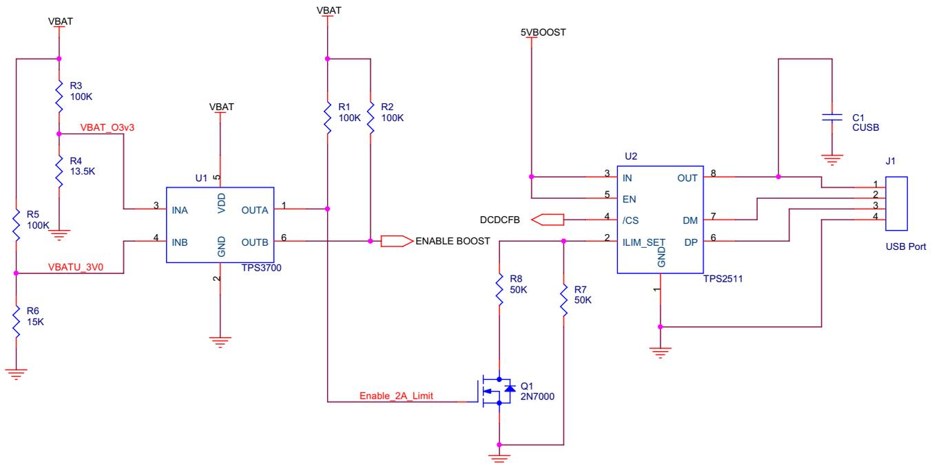
**Figure 4. Dynamically Adjusted Current Limit Based On Battery Voltage**
