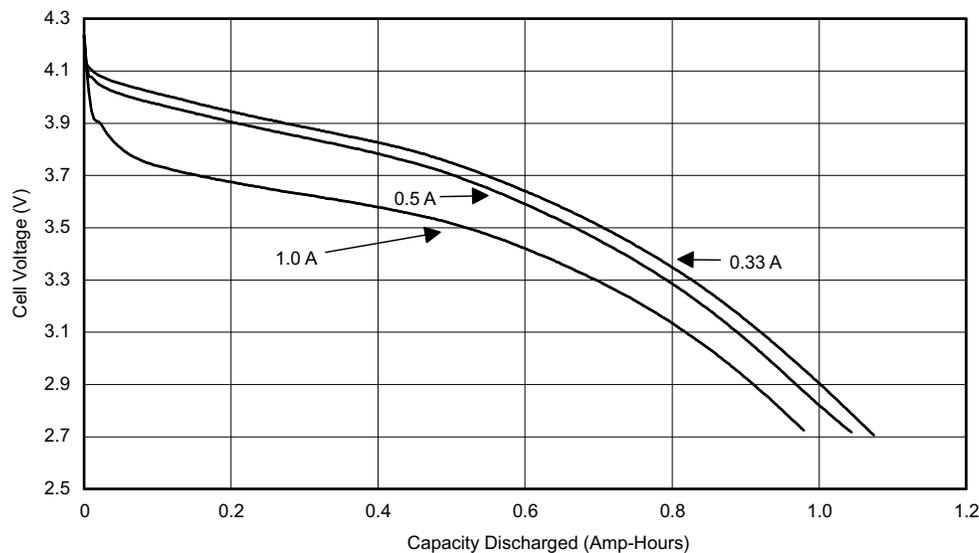
**Figure 5. Apparent Voltage vs Discharge Rate**
