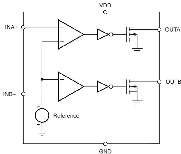
**Figure 2. TPS3700 Block Diagram**
