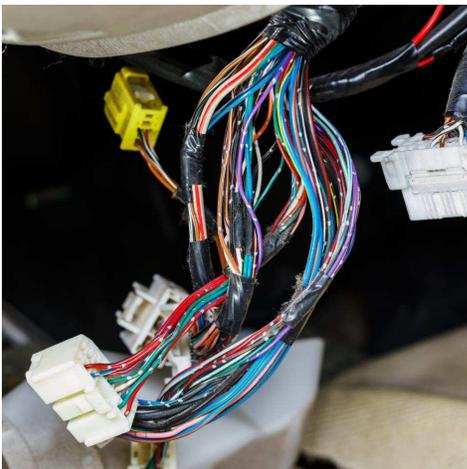
**Figure 1. Typical wiring harness found in a vehicle**
