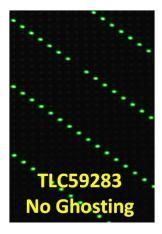
Figure 11. TLC59283 Eliminates Ghosting with Pre-charge FET
