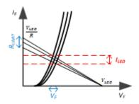
Figure 6. LED I-V Characteristics and Non-constant LED Current Solution
