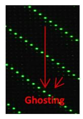
Figure 7. Ghosting Phenomenon in Time-multiplexing Circuit
