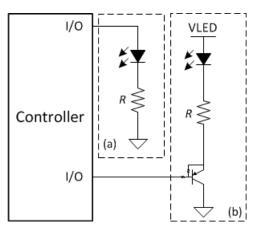
Figure 3. LEDs Directly Driven by I/Os
