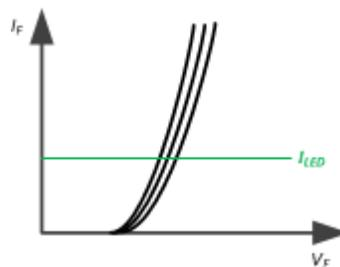
**Figure 9. TLC59283 Ensures Constant Current for Fetter LED Brightness Uniformity**
