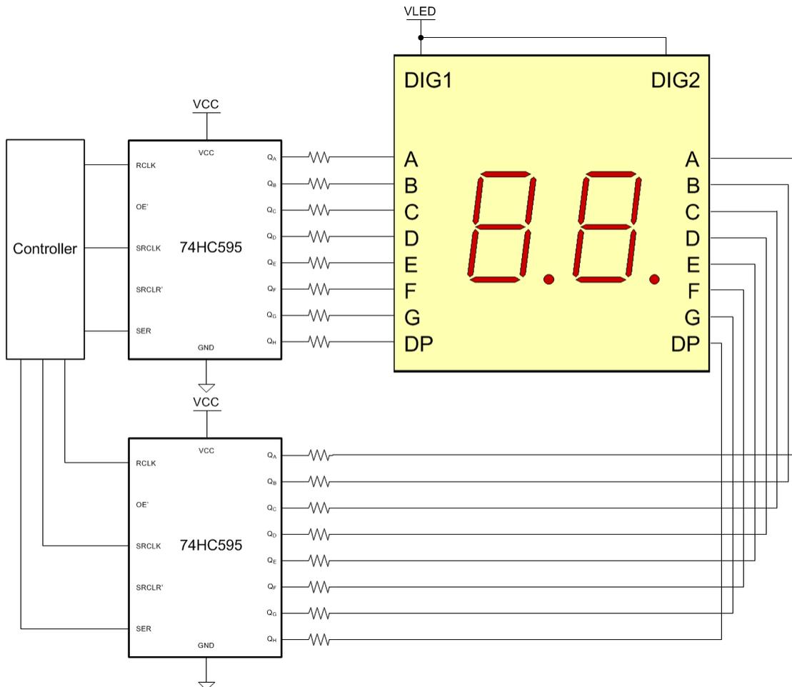
Figure 4. Two Seven-segment Displays (16 LEDs) Controlled by Shift Registers
