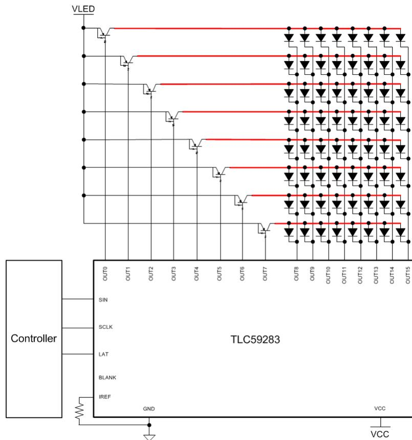
**Figure 13. Time-multiplexing Circuit Using TLC59283 and Less I/Os**
