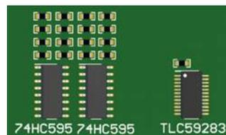
**Figure 10. TLC59283 Offers a Smaller PCB Size than Shift Registers**
