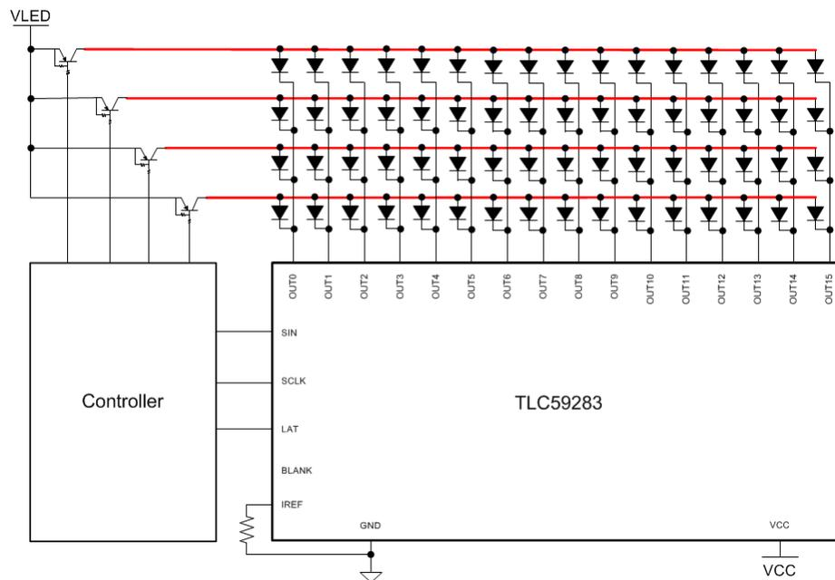
**Figure 12. Time-multiplexing Circuit Using TLC59283 and Enough I/Os**
