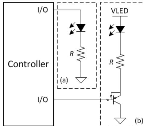
Figure 3. LEDs Directly Driven by I/Os
