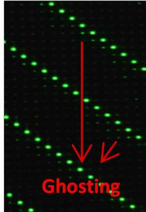
**Figure 7. Ghosting Phenomenon in Time-multiplexing Circuit**
