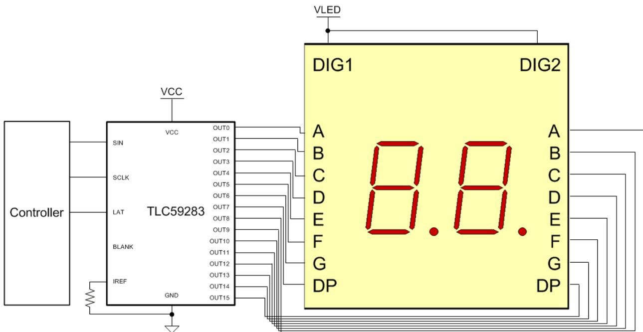
**Figure 8. Use TLC59283 to Drive Two Seven-segment Displays (16 LEDs)**
