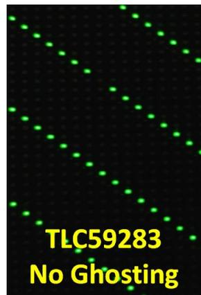
Figure 11. TLC59283 Eliminates Ghosting with Pre-charge FET
