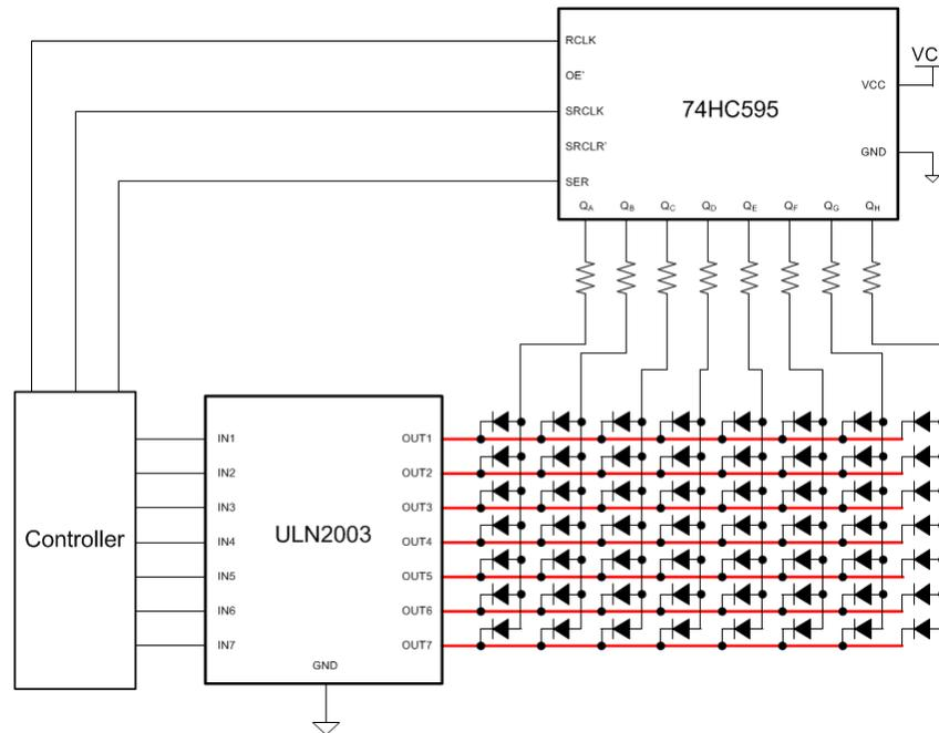
**Figure 5. Time-multiplexed LED Matrix by Shift Registers and Transistor Arrays**
