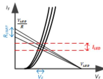
**Figure 6. LED I-V Characteristics and Non-constant LED Current Solution**
