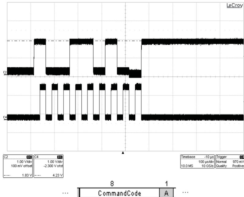
The second byte of I<sup>2</sup>C protocol contains the type of write/read (byte write) and register's address (1axh) where the operation is performed. C2 is SDA and C4 is SCL. The CDCE949 (slave) gives back acknowledgment after the last bit was patterned; only after the SCL last falling edge, the I<sup>2</sup>C bus is released to handle the next block of communication.
