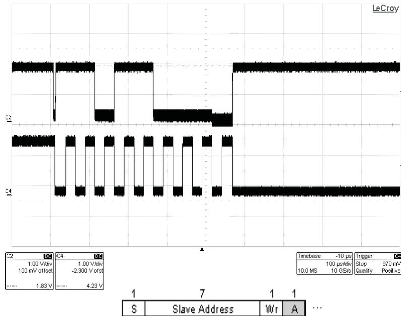
The first byte of the I<sup>2</sup>C protocol contains the device's slave address (1101100xb) and type of operation (0 = write). C2 is SDA and C4 is SCL. The CDCE949 (slave) gives back acknowledgment after the last bit was patterned; only after the SCL last falling edge, the I<sup>2</sup>C bus is released to handle the next block of communication.
