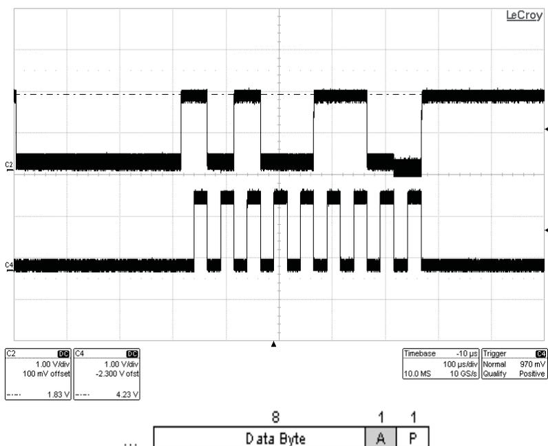
Data byte contains byte to write/read (A6xh).
