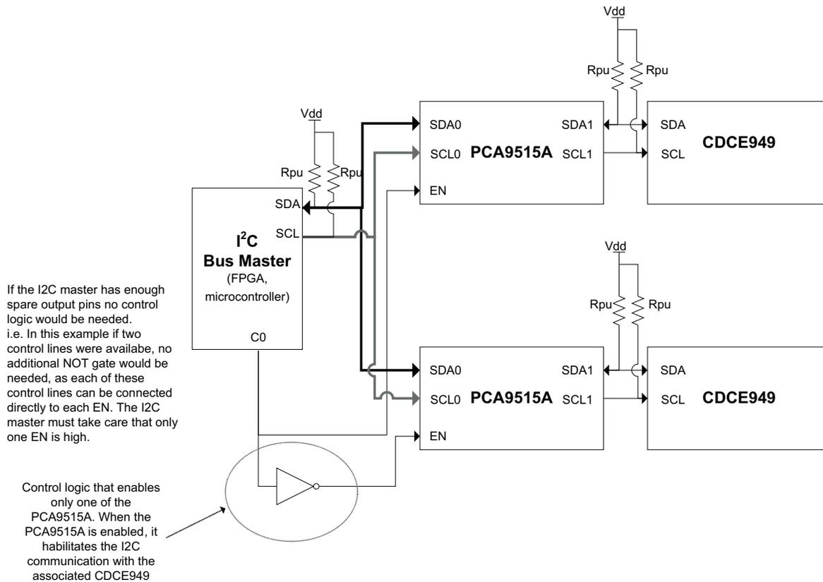
**Figure 6. Slave Address Conflict Solved With Bidirectional I<sup>2</sup>C Buffer**
