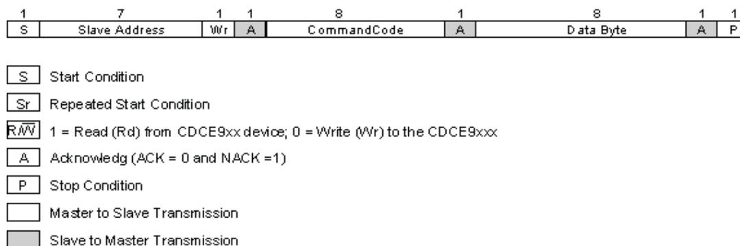
**Figure 1. I<sup>2</sup>C Programming Sequence for the CDCE949**
