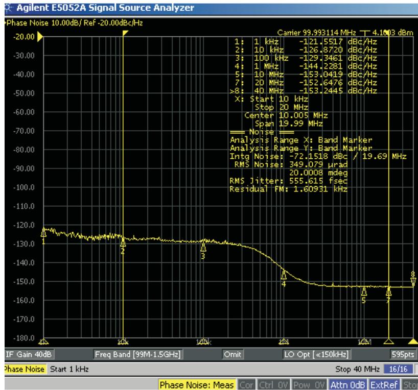
Figure 8. Phase Noise Performance of 100 MHz Clock Output with 25 MHz Crystal and 520 kHz PLL Loop Bandwidth
