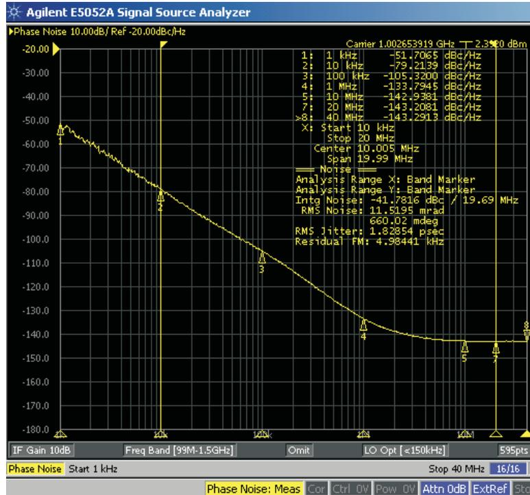
Figure 5. 1000 MHz Free Running VCO Phase Noise Performance
