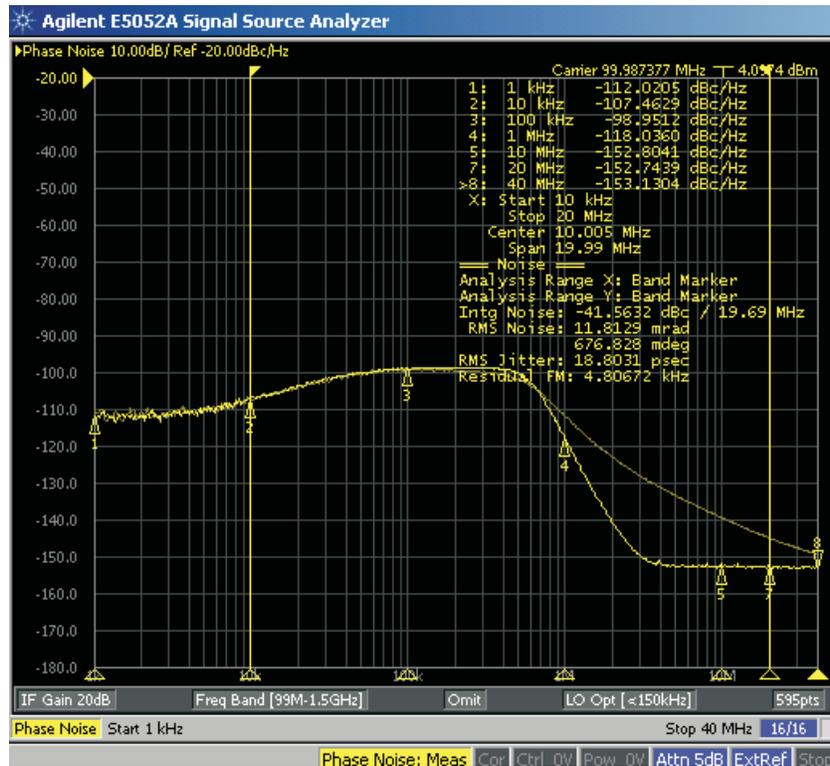
Figure 13. PLL Phase Noise Performance With 100 MHz Noisy Input Clock (520 kHz PLL Loop Bandwidth)
