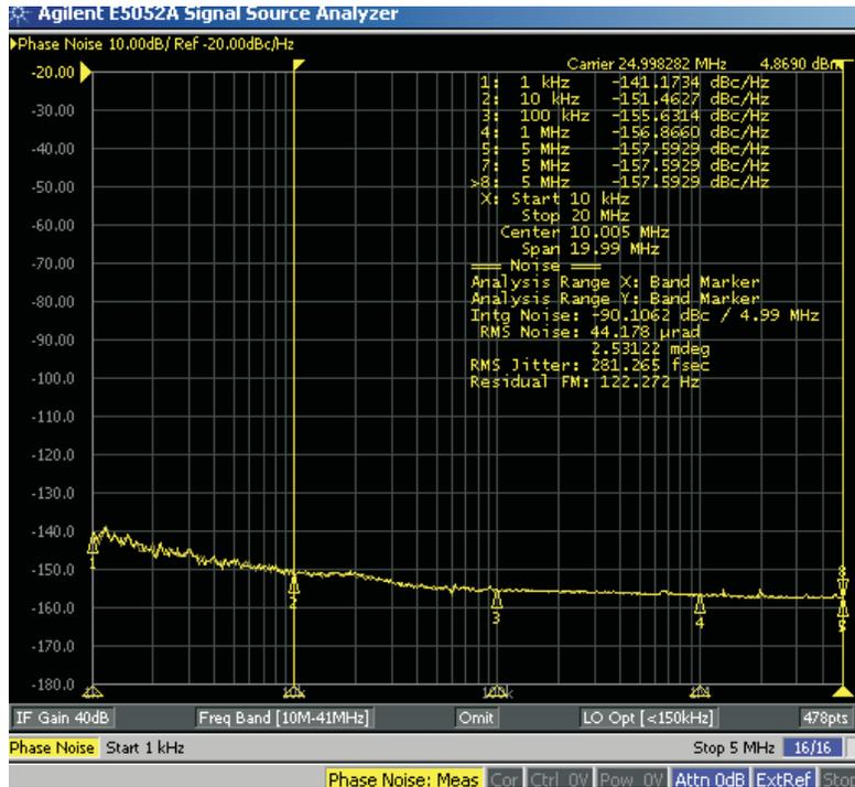
Figure 4. Phase Noise Performance of a Common Crystal and CDCE62005 Internal Oscillator
