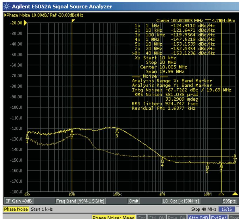
Figure 12. PLL Phase Noise Performance with 100 MHz Input Clock (105 kHz PLL Loop Bandwidth)
