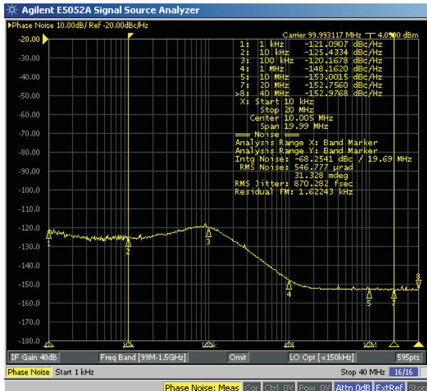
Figure 9. Phase Noise Performance of 100 MHz Clock Output with 25 MHz Crystal and 105 kHz PLL Loop Bandwidth
