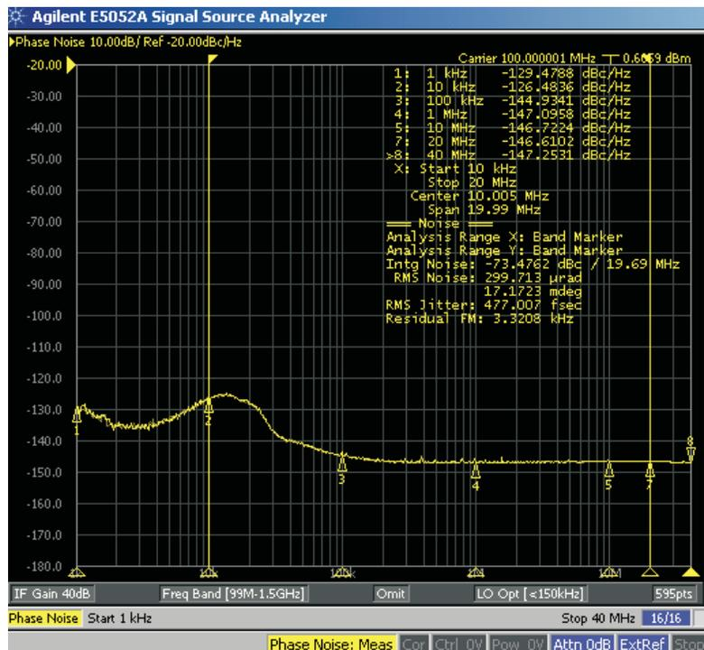
Figure 2. Phase noise Performance of a Typical Source (Agilent +HP8133)
