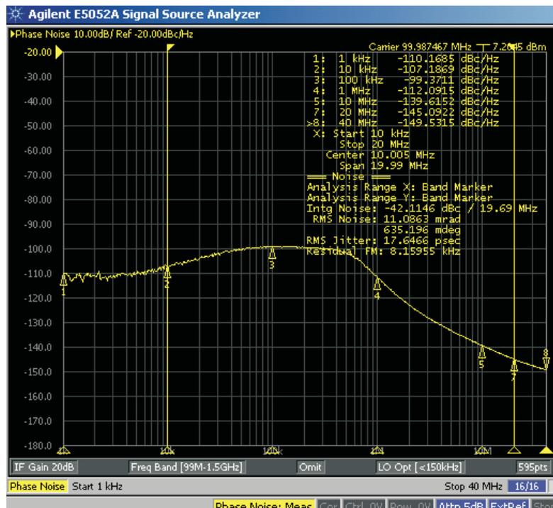
Figure 3. Phase Noise Performance of a Noisy PLL
