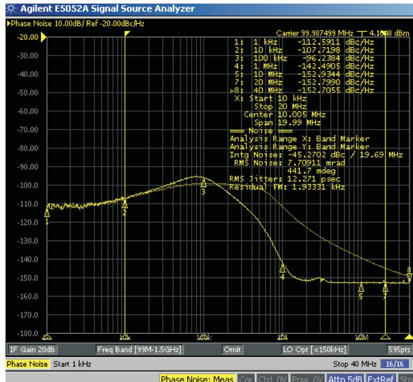
Figure 14. PLL Phase Noise Performance With 100 MHz Noisy Input Clock (100 kHz PLL Loop Bandwidth)
