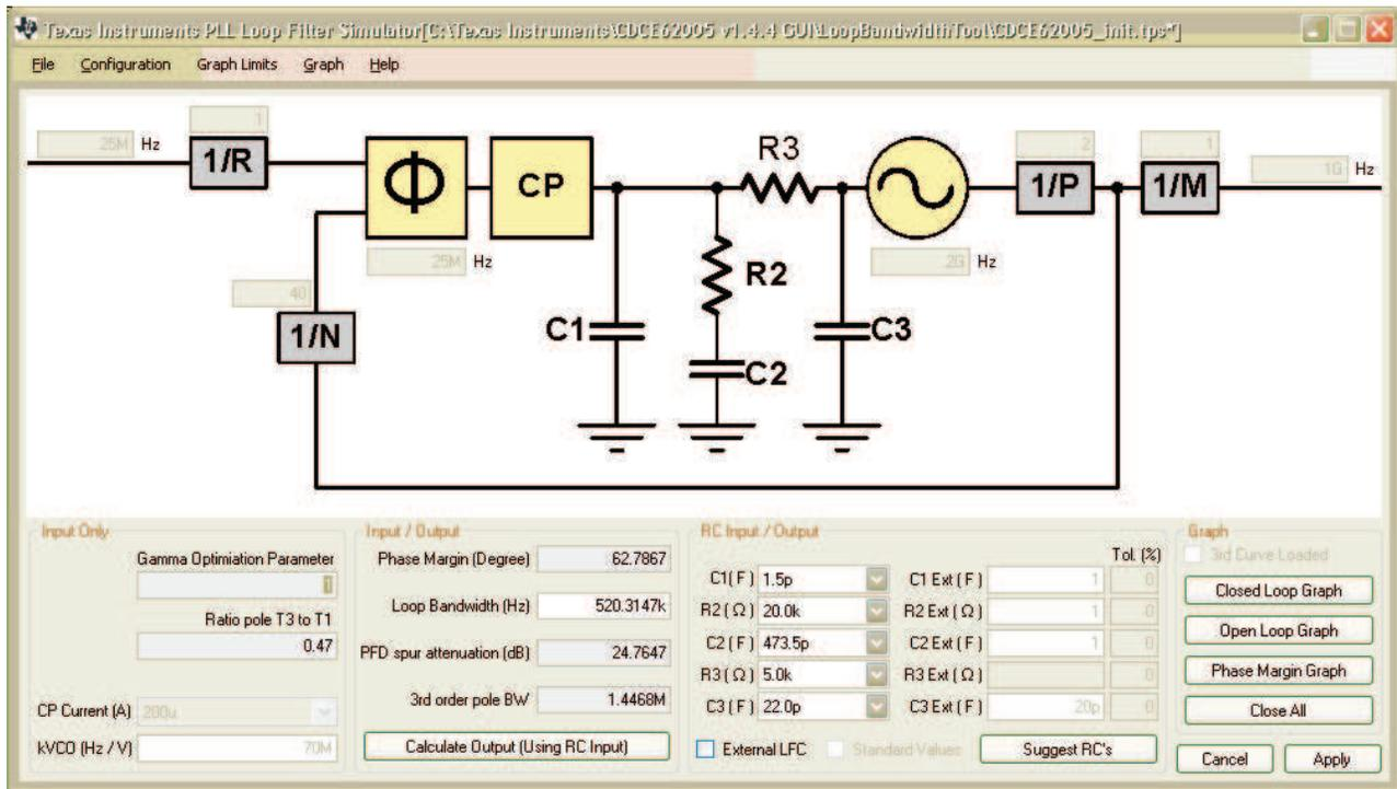
Figure 7. PLL Loop Bandwidth Calculation at 520 kHz
