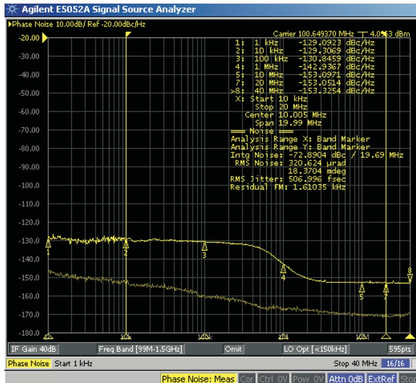
Figure 10. PLL Phase Noise Performance with 100 MHz Clean Input Clock
