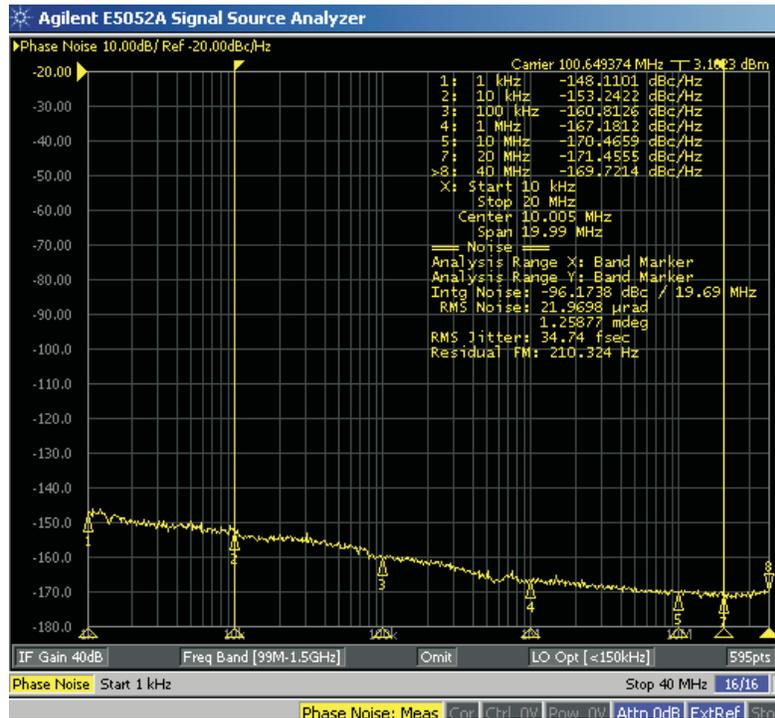
Figure 1. Phase Noise Plot of 100 MHz Generated from a Clean Clock Source (Wenzel Oscillator)
