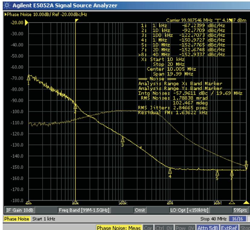
Figure 15. PLL Phase Noise Performance With 100 MHz Noisy Input Clock (440 Hz PLL Loop Bandwidth)
