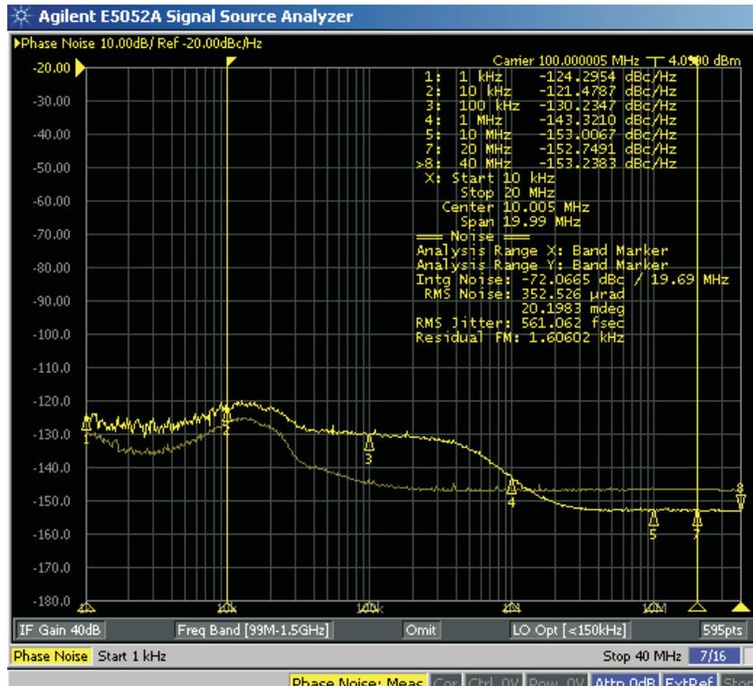
Figure 11. PLL Phase Noise Performance with 100 MHz Input Clock (520 kHz PLL Loop Bandwidth)
