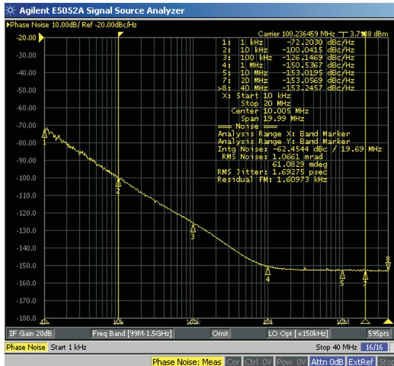
Figure 6. 100 MHz Free Running VCO Phase Noise Performance
