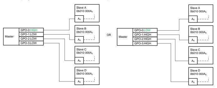
Figure 5. Example of GPOs Controlling Addresses to Communicate with Slave A
