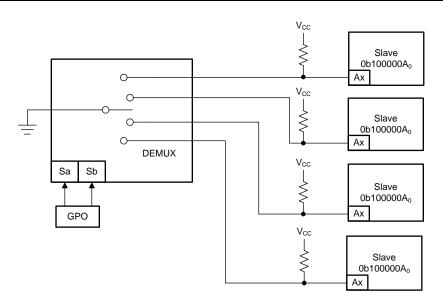
Figure 6. Example of GPO Controlling a MUX
