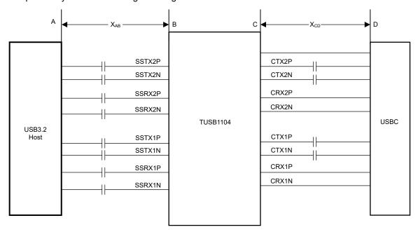
Figure 2-1. Typical USB 3.2 Gen2x2 Application with TUSB1104
