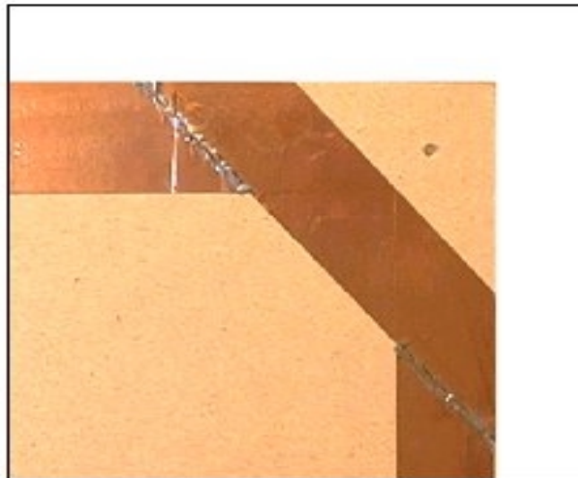
Figure 1. Copper tape folded and soldered
