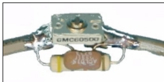
Figure 15. Small Round Antenna Tuning circuit
