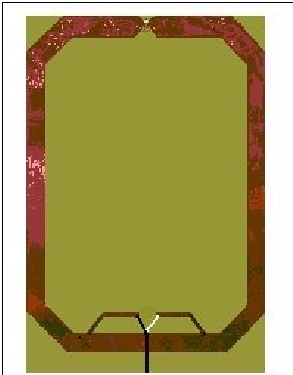
Figure 7. Tape Antenna (550mm x 800mm)
