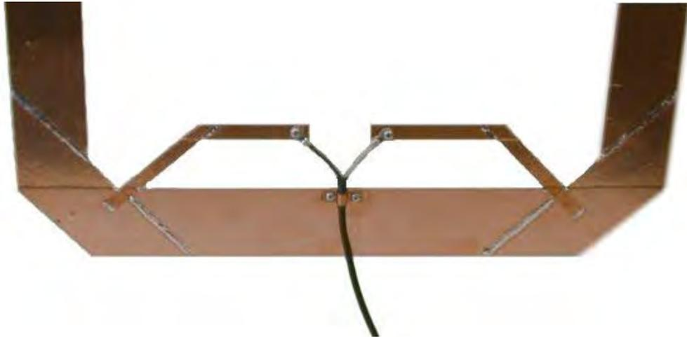
**Figure 18. T-Matched Tape Antenna**
