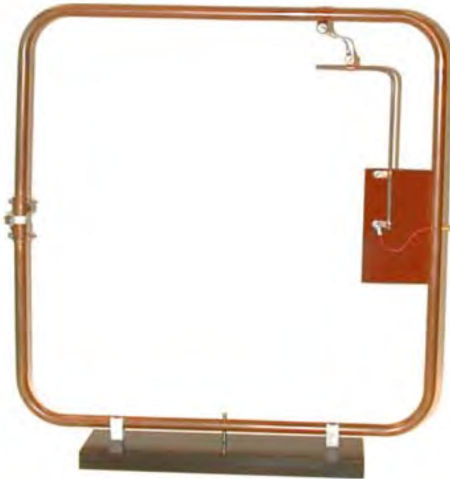
**Figure 14. Gamma Matched Antenna**
