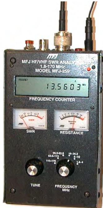
Figure 2. Antenna Analyzer
