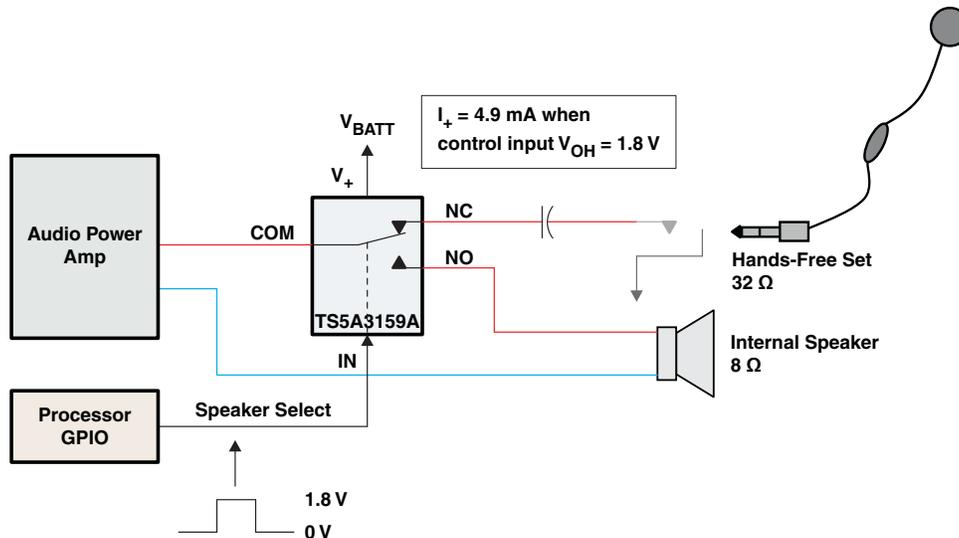
Figure 5. Excess Current Consumption – Control Input Is at Lower Voltage Than  $V_+$
