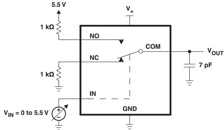
Figure A-1. Test Setup for TS5A12301E ( $V_{OUT}$  vs  $V_{IN}$ )
