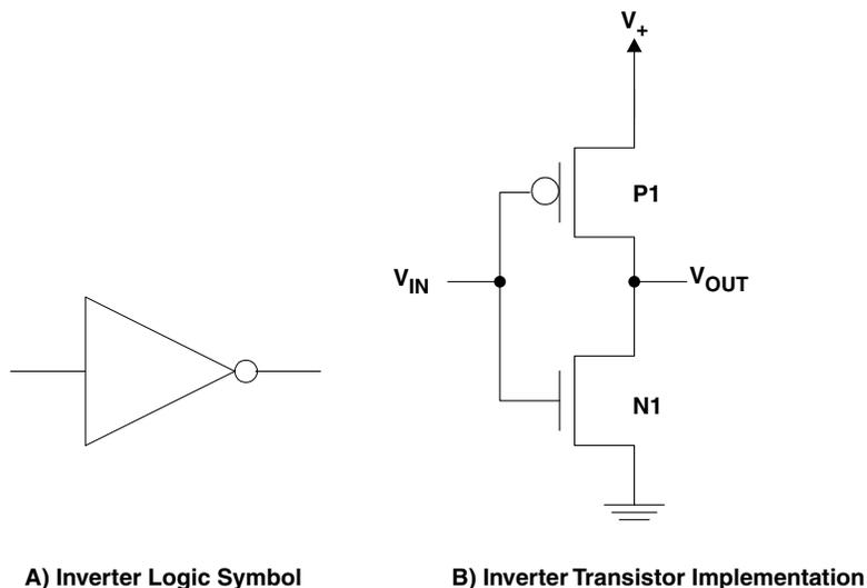
Figure 2. Simple CMOS Inverter
