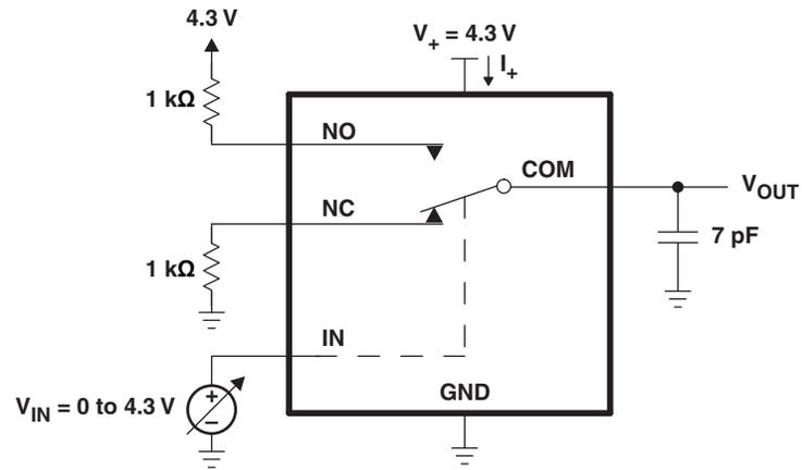
Figure A-3. Test Setup for Supply Current vs Control Input Voltage
