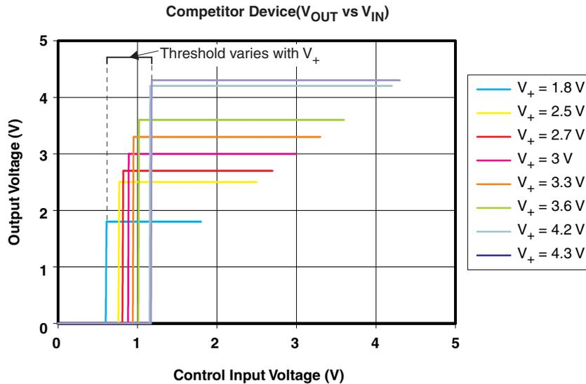
Figure 9. Input Threshold Variation on Competitor Device
