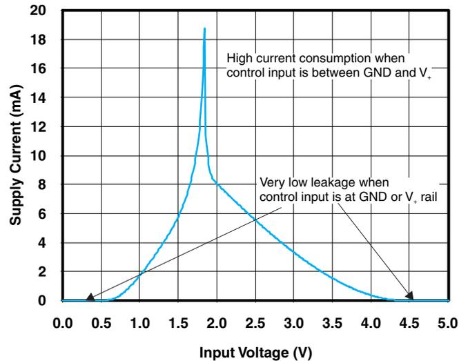
Figure 1. Supply Current vs. Control Input Voltage for the TS5A3159A ( $V_+ = 5\text{ V}$ )
