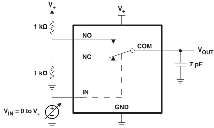
Figure A-2. Test Setup for Competitor Device ( $V_{OUT}$  vs  $V_{IN}$ )
