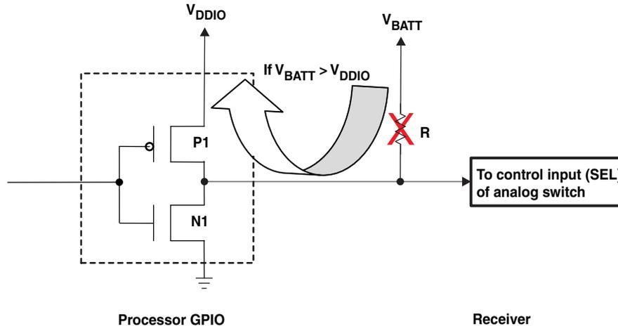
**Figure 6. Drawbacks of Using a Pullup Resistor Directly From Processor GPIO to  $V_{BATT}$  for Up-Translation**
