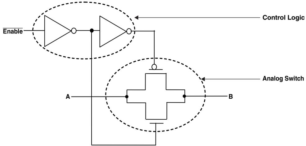
Figure 3. Internal Structure of a Typical Analog Switch
