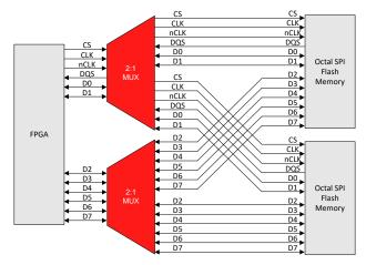
Figure 5. FPGA Access to Multiple Octal SPI Flash Memories
