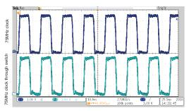
Figure 6. 75-MHz Clock Passing Through TMUX1574
