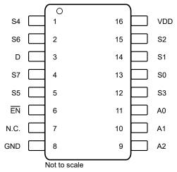
Figure 4-2. Pin Diagram (SOT-23-THIN) Package
