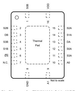
Figure 4-6. Pin Diagram for TMUX1309-Q1 in WQFN Package
