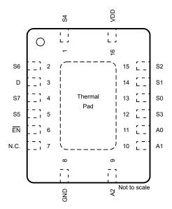
Figure 4-3. Pin Diagram for TMUX1308-Q1 in WQFN Package
