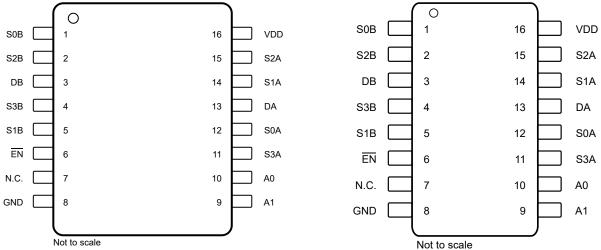
Figure 4-4. Pin Diagram (TSSOP) Package
