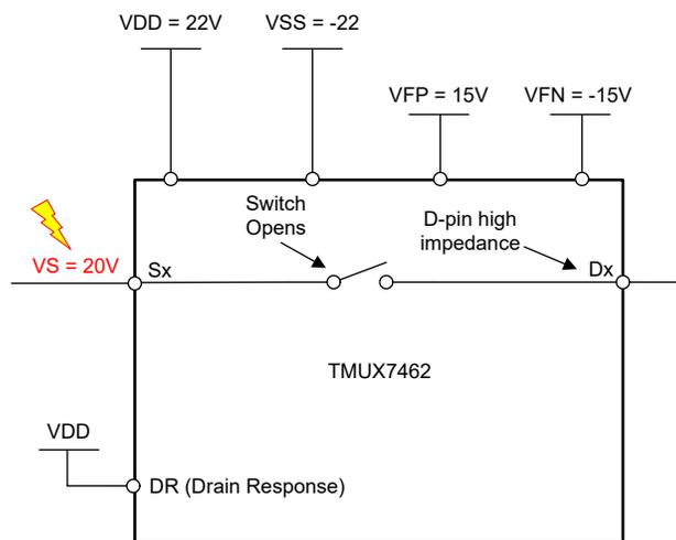
**Figure 2-4. TMUX7462F Drain Response tied to VDD**
