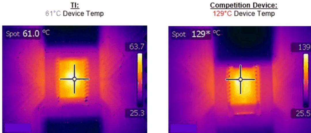
**Figure 2-6. TI Device vs. Competitor Device**
