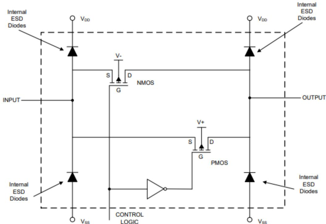
**Figure 1-1. CMOS Switch Architecture**
