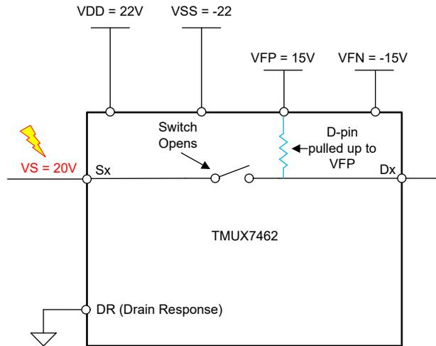
**Figure 2-3. TMUX7462F Drain Response tied to GND**
