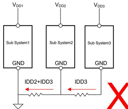
Figure 1-5. Improper Grounding and Effects
