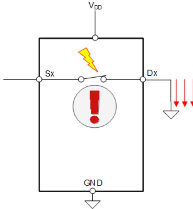
Figure 1-4. Short Circuit Fault
