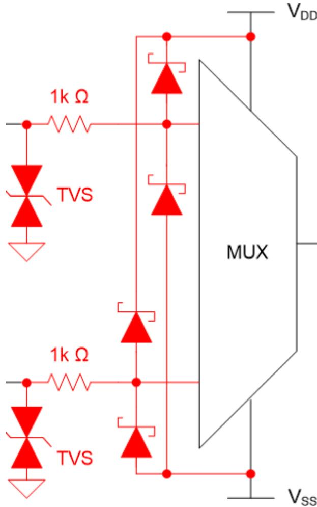
**Figure 2-7. Mux without Integrated Fault Protection**
