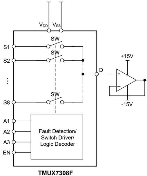
**Figure 2-1. Main Supply Fault Control**
