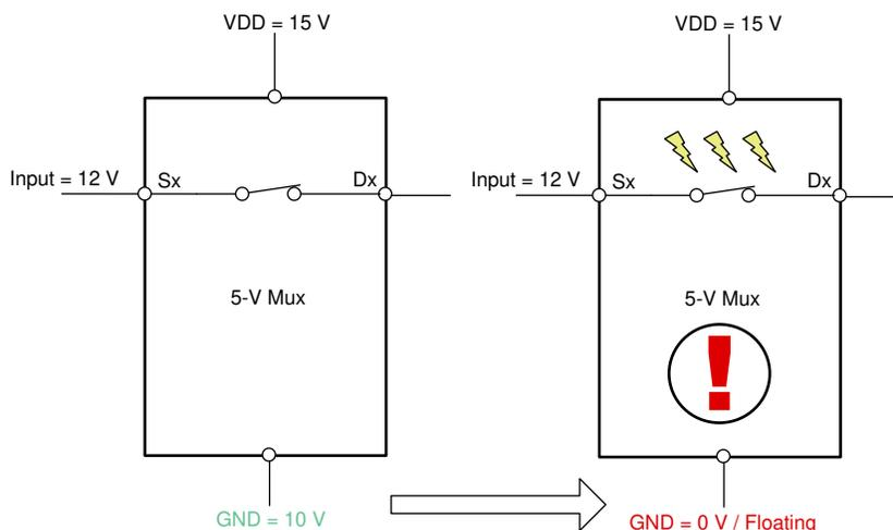
Figure 1-7. Common Mode Fault
