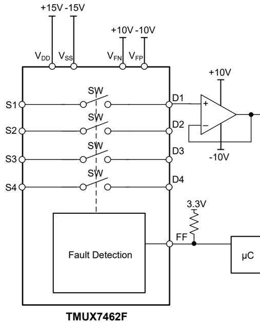
**Figure 2-2. Secondary Supply Fault Control**
