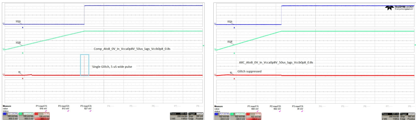
Figure 5. Competition (0.8 V) vs AXC (0.65 V), Slow Output Ramp 0.8 s (1 s/V) With 0-V Input
