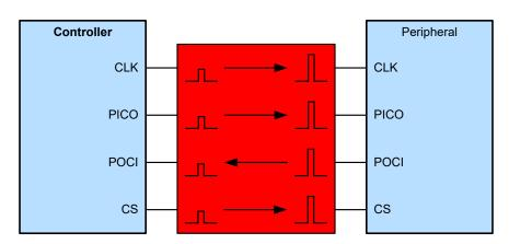
**Example SPI Voltage Translation Block Diagram**
