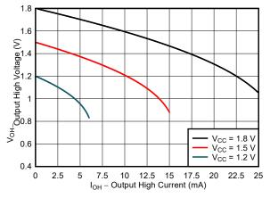
Figure 2-5. Typical ( $T_A$ =25°C) Output High Voltage ( $V_{OH}$ ) vs Source Current ( $I_{OH}$ )
