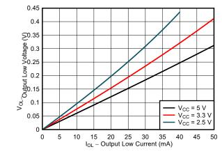
Figure 2-6. Typical ( $T_A$ =25°C) Output High Voltage ( $V_{OL}$ ) vs Sink Current ( $I_{OL}$ )
