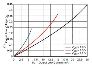
Figure 2-7. Typical ( $T_A$ =25°C) Output High Voltage ( $V_{OL}$ ) vs Sink Current ( $I_{OL}$ )
