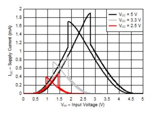
Figure 2-3. Supply Current Across Input Voltage (2.5 V, 3.3 V, and 5 V Supply)
