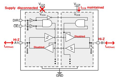
Figure 3-1. V<sub>CC</sub> Disconnect Feature
