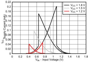
Figure 2-2. Supply Current Across Input Voltage (1.2 V, 1.5 V, and 1.8 V Supply)
