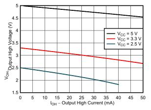
Figure 2-4. Typical (T<sub>A</sub>=25°C) Output High Voltage (V<sub>OH</sub>) vs Source Current (I<sub>OH</sub>)
