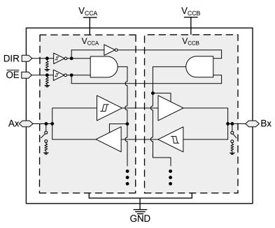
Figure 2-1. LXC I/O and Control Input Circuitry
