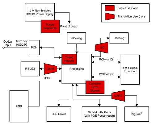
Figure 1. Simplified Block Diagram for Optical Network Terminal Units
