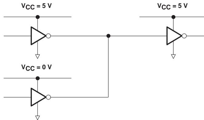
**Figure 4. Partial Power Down With Bus Drivers**
