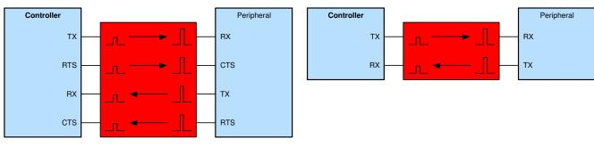
Figure 2. Using Voltage Translation With the UART 4-Wire Communication Bus Figure 3. Using Voltage Translation With the UART 2-Wire Communication Bus
