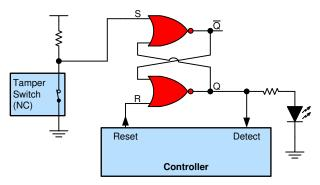
Figure 7. Using Logic to Monitor a Normally Closed (NC) Tamper Switch
