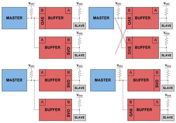
Figure 17. All Possible Buffer Combinations that are Allowed and Not Allowed (red cross).
