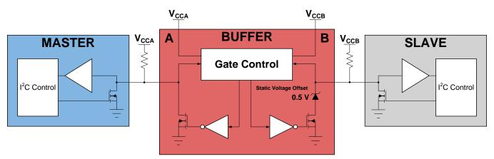
Figure 12. Example of a Buffer That has a Static Voltage Offset That is on the "B" Side of the Buffer
