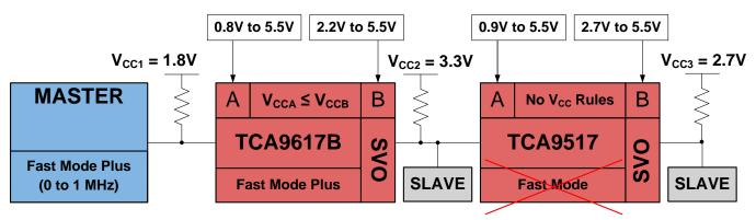
Figure 23. TCA9517 Does not Support Fast Mode Plus
